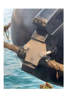
S&S Floats have developed a metal clamp that eliminates the need for rope lashing and ensures the floats stay secure on the farm.
