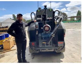
A LiDAR (Light Imaging, Detection and Ranging) unit on each OXIN uses laser beams to detect gaps in rows, look for obstacles, and ensure implement arms are in the right place. On-board sensors gauge pressure and levels of water and spray. They automatically stop if there is an issue.
